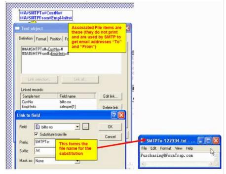
"billto no" is inserted between prefix and suffix to give file name: SMTPTo-122334.txt (for Customer 122334), content is the email address of the client.
